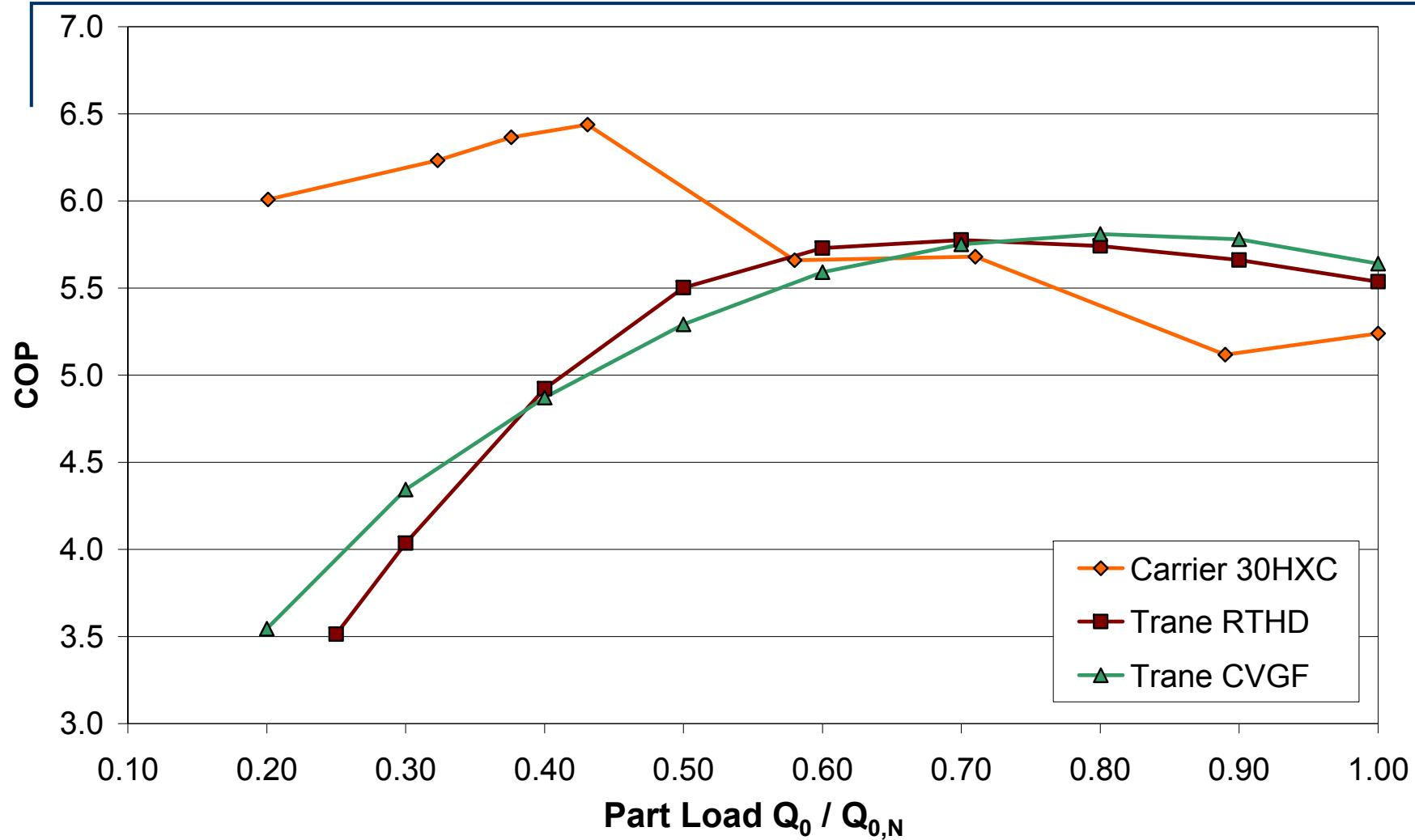
Cold water: 6 / 12 °C, Cooling water: 26 / 32 °C
