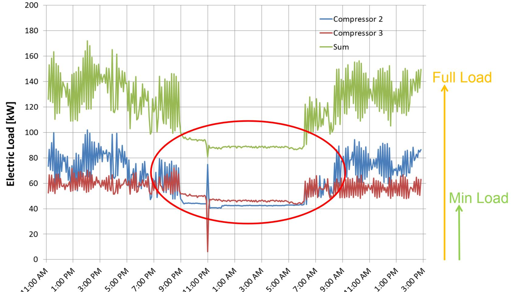
**Single Compressor rated at 136 kW on load. Min Load Variable Speed 30 %**
