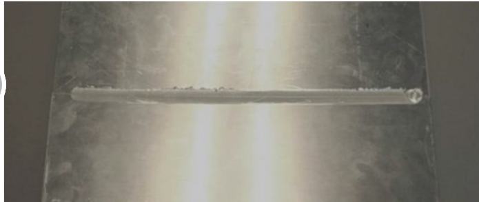
2,3-mm 2024-T3 Butt weld
