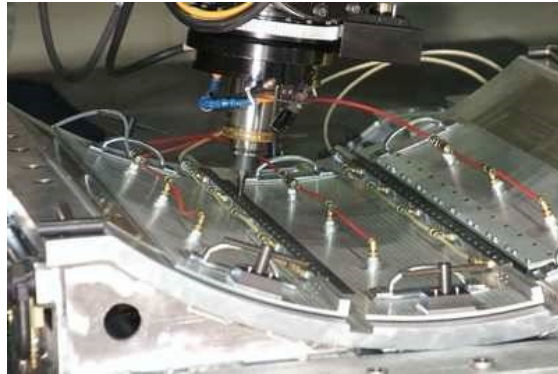
welding of fuselage of the Eclipse 500 Business Jet
